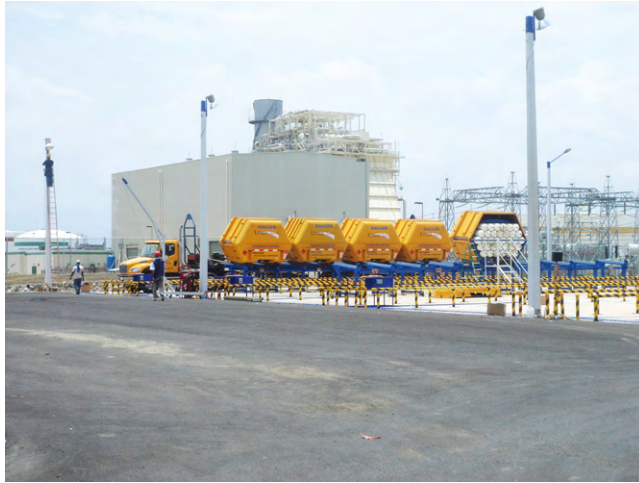
Microbox hooks up to pipeline or AD installation to MAT transport modules - Galileo Argentina
