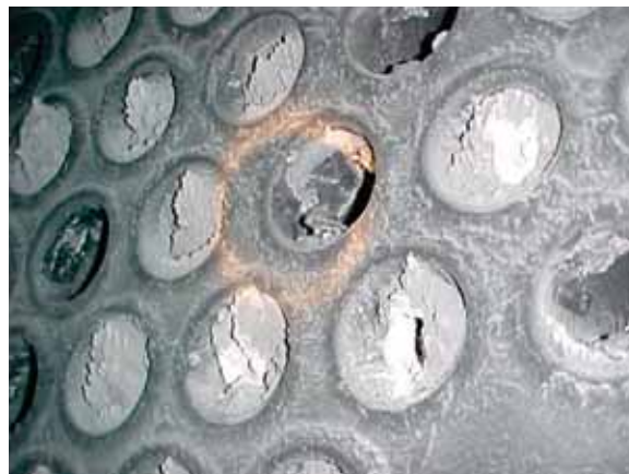
Figure 1-7 Formation of Deposits on Boiler Tubes (Boiler Fouling & Deposits)
