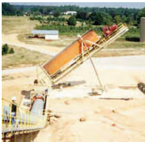
Figure 2.8 Trailer Tipper Unloading Biomass
