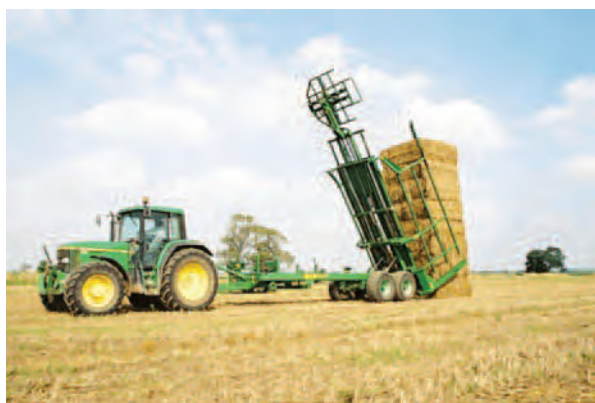
Figure 2.3 Bale Accumulator Used to Aggregate Bales in the Field
