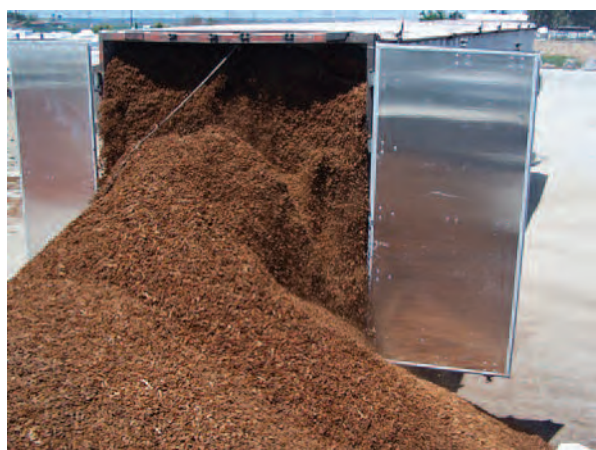
Figure 2.6 Unloading Biomass from a Walking Floor Trailer
